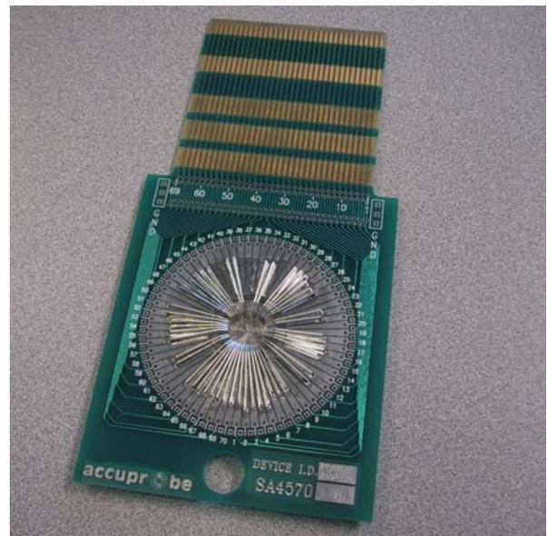
protect the probe card's surface from contaminants. Every probe card is reinforced with a stiffener that is laminated to the underside of the probe card. This attention to design, construction and electrical performance separates Accuprobe cards from the competition.
